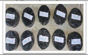
Figure 7(b). Specimens prepared for sorptivity test
