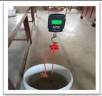
Figure 6(a) Specimens in the boiling water (b) Measuring apparent weight of the specimen
